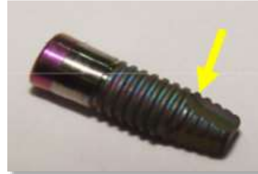
Commercial titanium screw with nanosized hydroxyapatite coating (100 nm)
